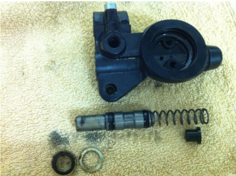
Next you can prepare the new master piston that should look just like your old one in terms of parts. Make sure you keep the old washer, seal and ring from the old piston; else you would have to make you a tool to mount the sucker:
