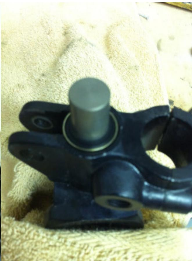
Next you can go two ways: either you find or make yourself a tube that has outer diameter =>20mm max (or 19mm) and inner diameter 13mm – 14mm max or you re-use (like I did) the old washer and seal to push the new one in with a piece of round material:
