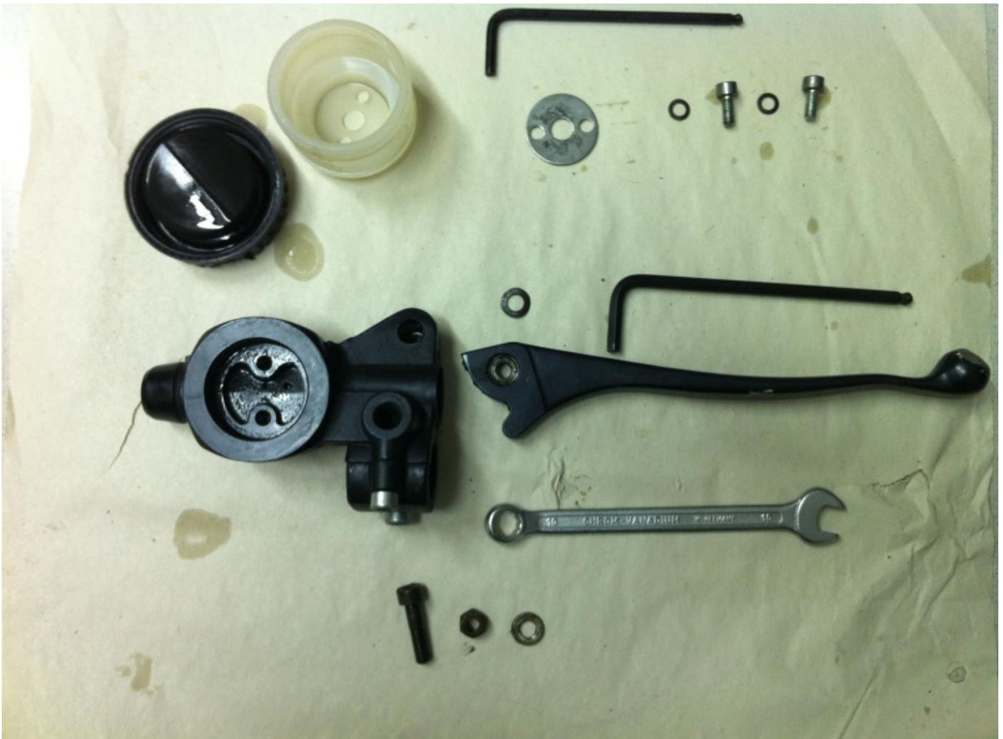
Now you need to dismount the master piston. For that you mount the master cylinder into the vise with an old towel or so to make sure you don't scratch the surface. Make sure you put the side up that takes the brake line and to put the side downwards that takes the lever (see next page). Don't over tighten the vise!! This is cast alloy, it might brake...
