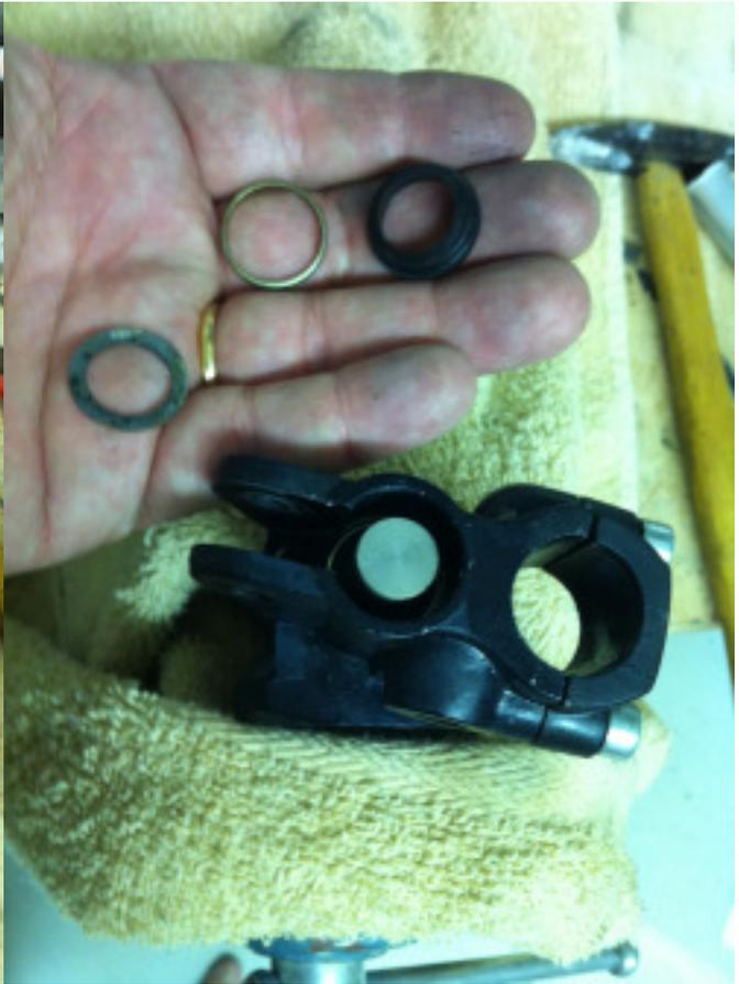
Piston should stay in the master. Time to mount the lever again, which you should have greased a bit. Don't forget the spring-washer that sits in the lever!!
