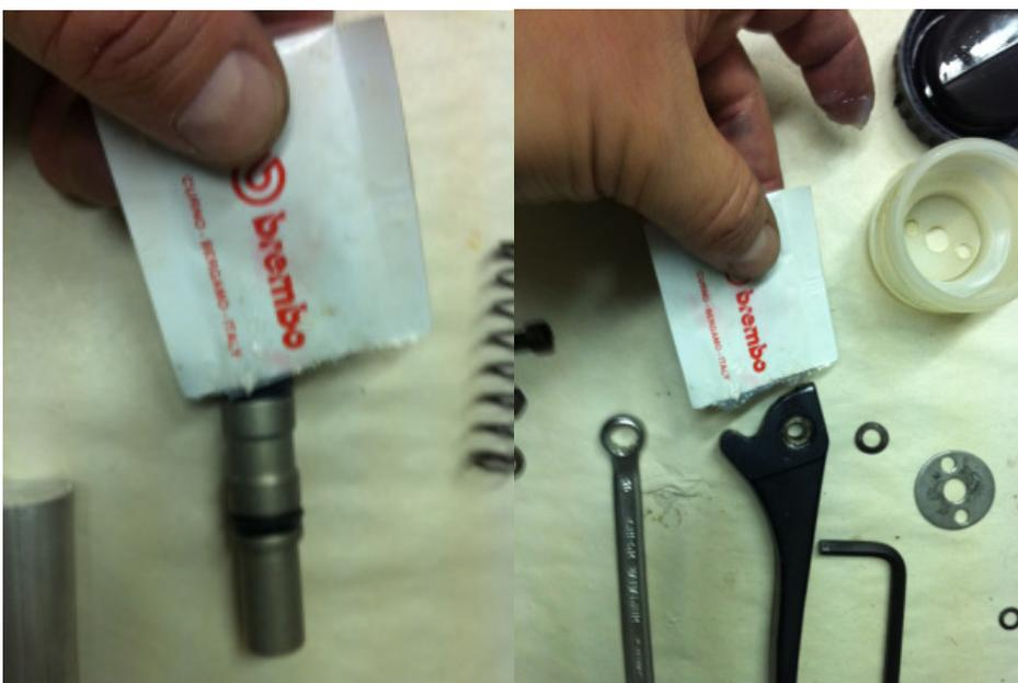
After that you put the spring on top of the piston so it stays there and put the plastic cap on top of the spring. This way you can put everything easily into the master.
