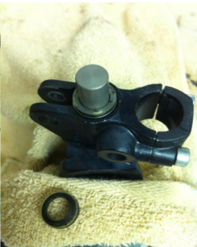
After you put everything on, you push the package down with the round material (or the tube) and give it a push or two with the hammer.
