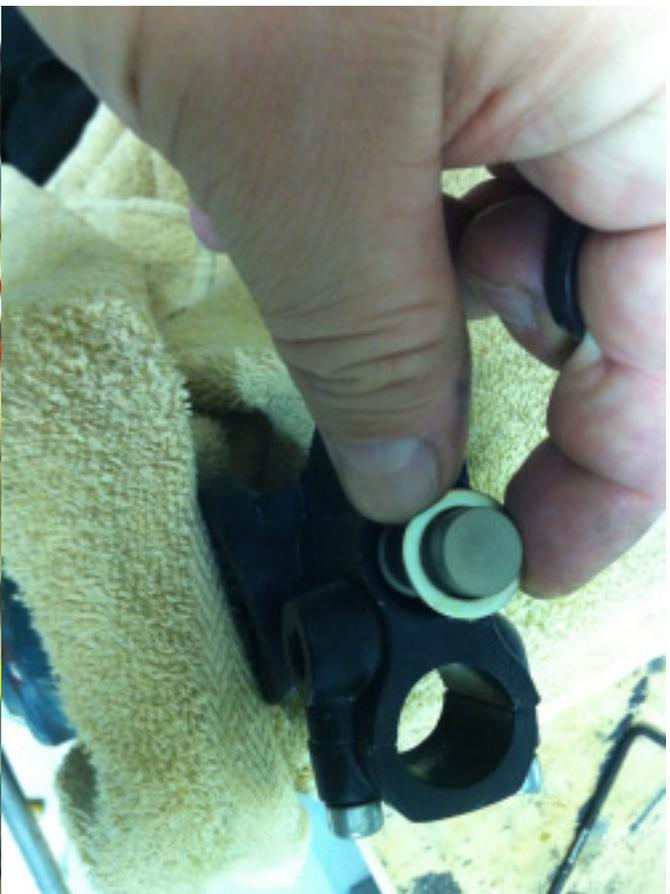
Make sure you take the parts the right direction!! Left side on these pics is DOWN. First put the brass ring with the SMALLER outer diameter over the rubber seal! At least that was how it was mounted on all my masters...
