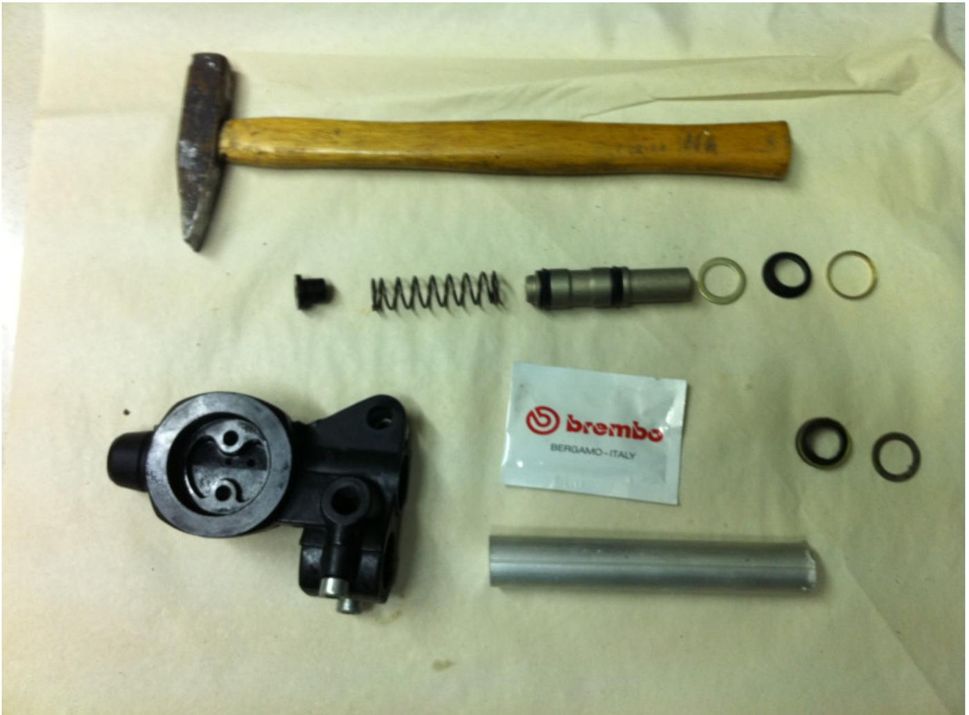
Now grease the sealing rubber lips of the master with the grease coming with the kit. Use some for the lever (below the washer and on the contact surfaces):
