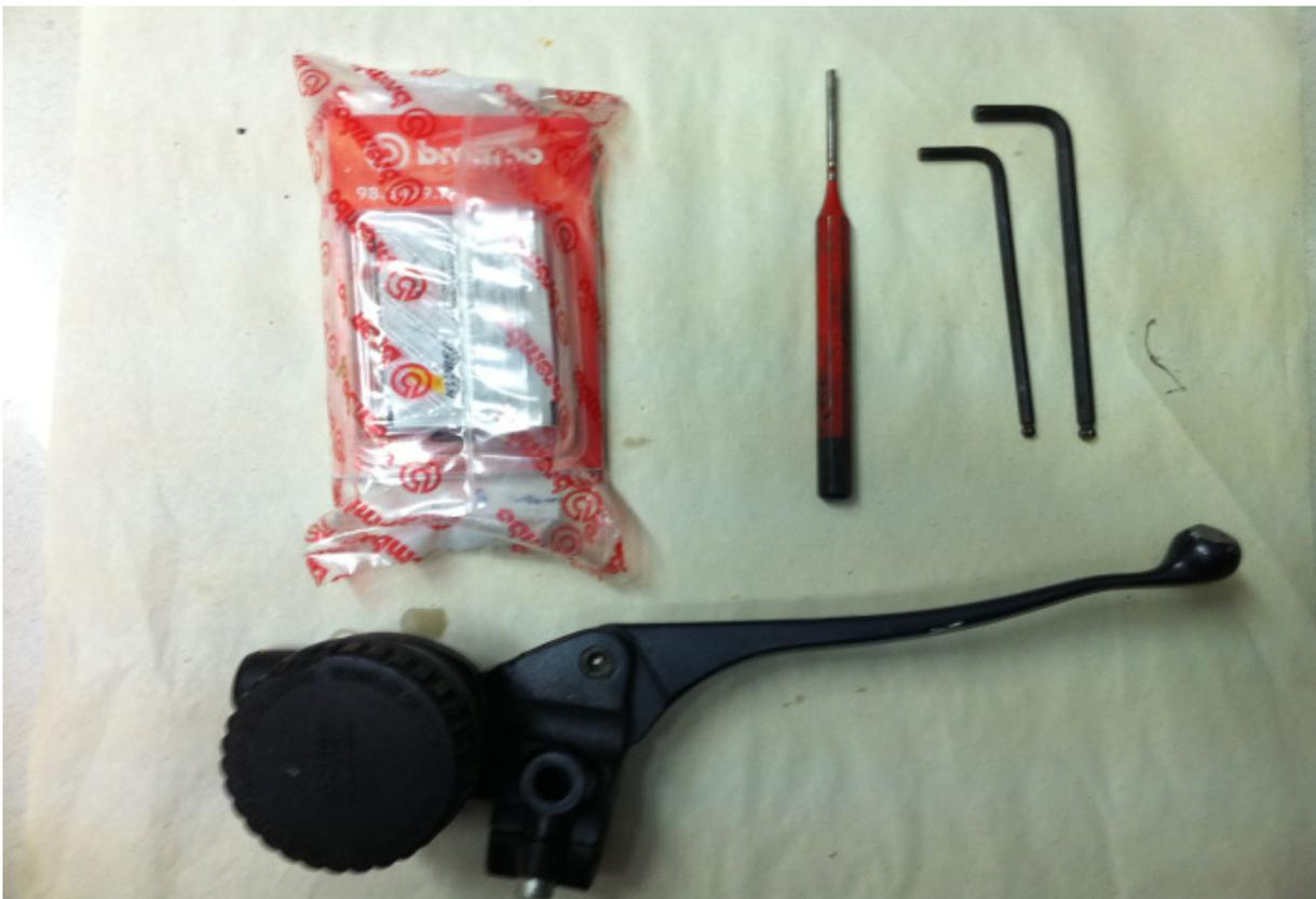
The reservoir is held by two screws and a plate only. Once the screws are removed, you can turn the plastic reservoir in its seat and gently pull it out. Time to dismount the lever by first removing the 10mm nut and then unscrew the Allen screw. Make sure you don't lose the little spring-washer on one side of the lever! Clean off old grease/dirt!
