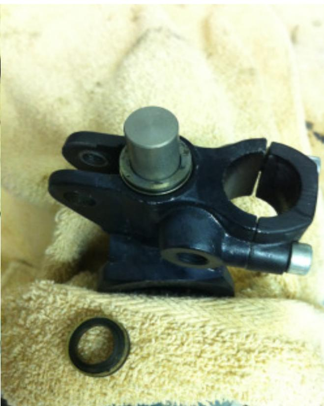
After you put everything on, you push the package down with the round material (or the tube) and give it a push or two with the hammer.
